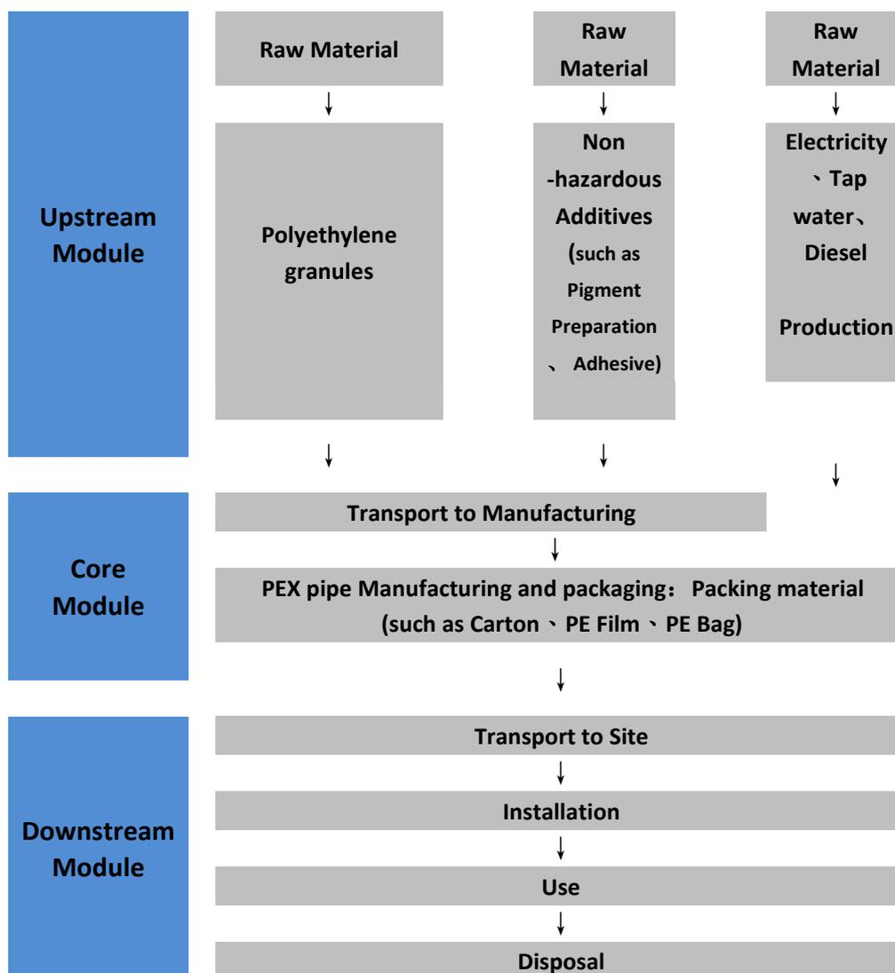
Figure 1 - life cycle diagram of PEX pipe production
