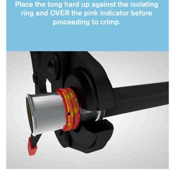
Complete the crimp by closing the tong. Open the tong and the pink indicator will break apart showing that the crimp has been completed. You only need to crimp once.
