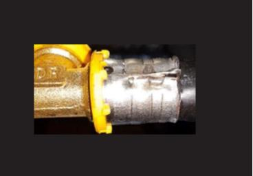
Crimp pinching can also occur when the tong has not been placed evenly on the sleeve. Water will leak through the pinched area.
