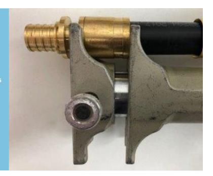
The completed compression joint will have the sleeve pulled all the way up to the face of the fitting as shown right.
