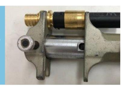
Operate the tool so that the sleeve is drawn over the pipe until it reaches the shoulder of the fitting.
