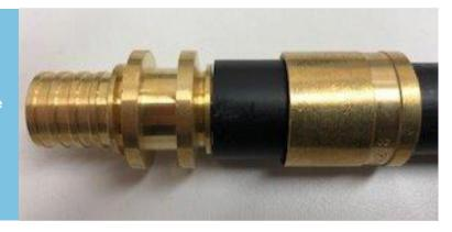
Sleeve has been placed with the bevel edge facing the wrong direction. You can tell it is the wrong direction by the indented ring on the sleeve.
