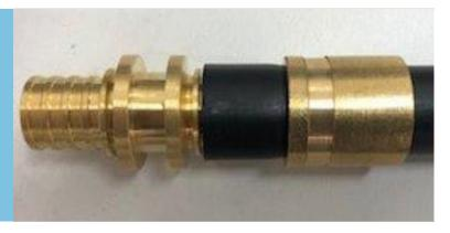
If you complete the joint with the bevel edge of the sleeve in the wrong direction the pipe will be pushed out at the face of the fitting. This may result in leakage and/or total failure of the joint over time.
